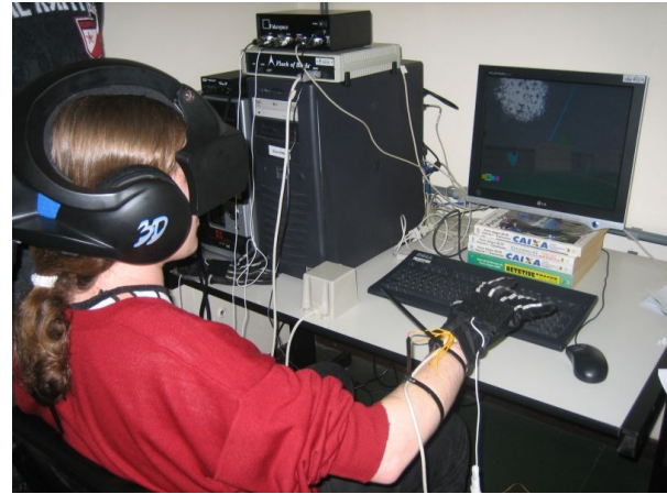
Figure 5: User playing GhostHunt with the proposed technique: he is wearing a head-mounted display, a pinch glove and a 3D tracker on his arm.
