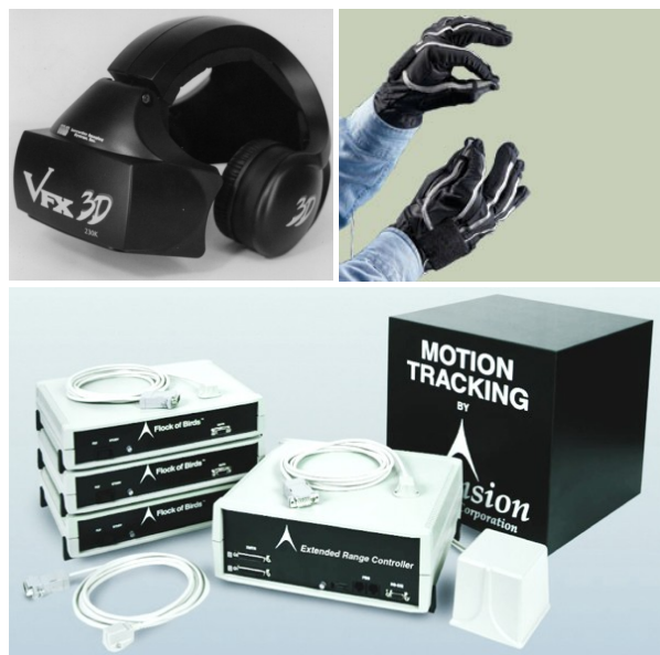
Figure 3: Devices used. Top-left: VFX3D (head-mounted display). Top-right: Pinch Gloves (data glove). Bottom: Flock of Birds (3D tracker).
